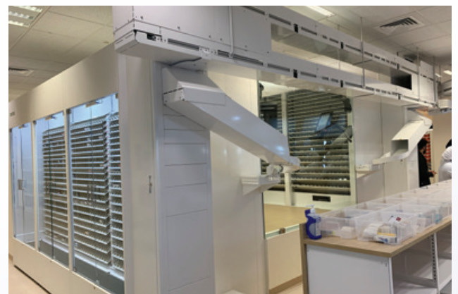
Automatic dispensing with CONSIS robots at Jaber Al Ahmad Hospital in Kuwait
