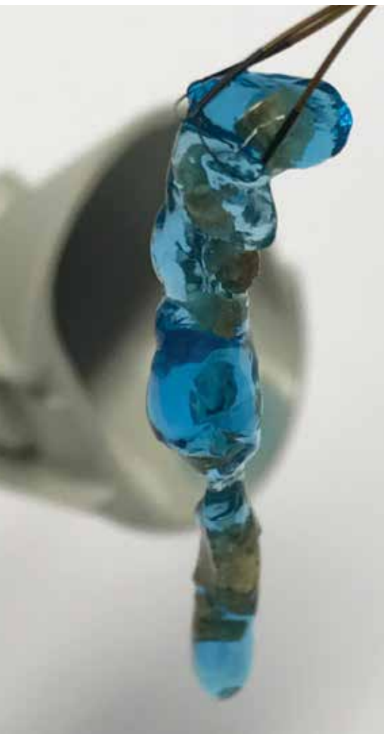
mediNiK® in use: the hydrogel with encapsulated kidney stone fragments following removal from the kidney.
