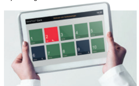
Ward terminal with room overview: An alarm was triggered in the room marked in red - someone fell here. Residents are active in the blue rooms, there is no activity in the green rooms.
