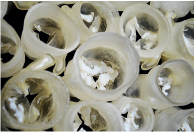
CT scans and a custom parametric modelling process were combined to create multi-material physical models of patients' aortic heart valves, each with its own unique size, shape, and amount of calcification.
