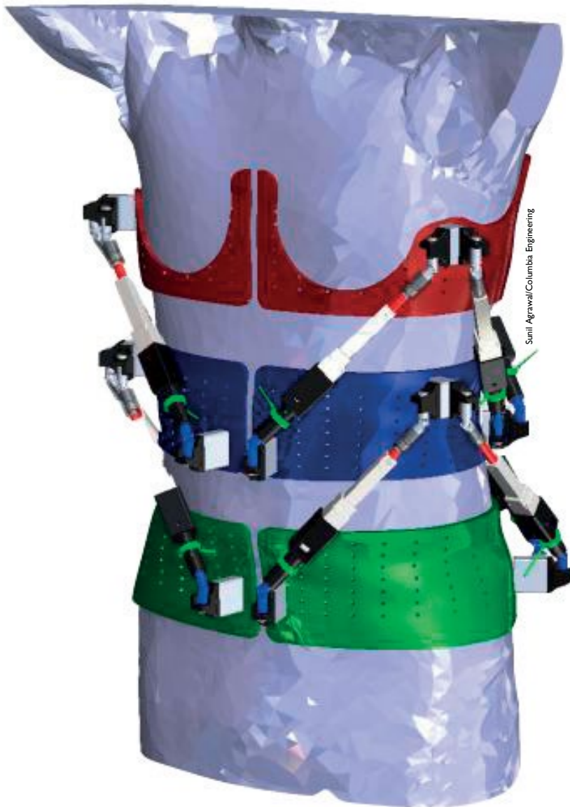
The Robotic Spine Exoskeleton consists of two six-degrees-of-freedom parallel-actuated modules connected in series, each with six actuated limbs. Each module controls the translations/rotations or forces/moments of one ring in three dimensions with respect to the adjacent ring.
