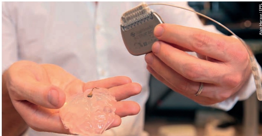
The brain-spine interface uses a brain implant like this one to detect spiking activity in the brain’s motor cortex. Seen here, a microelectrode array and a silicon model of a primate’s brain, as well as a pulse generator used to stimulate electrodes implanted on the spinal cord.
