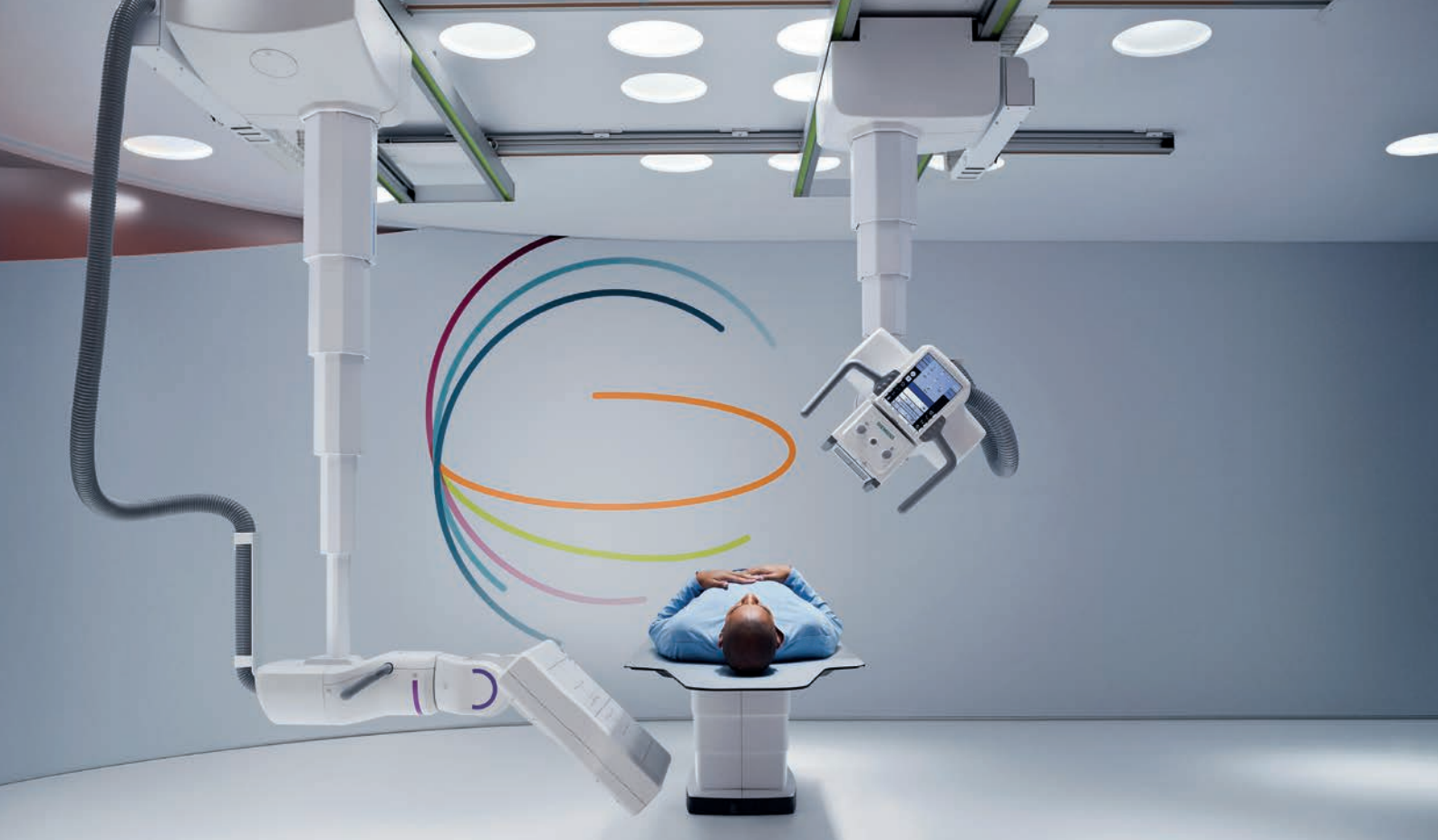
The two ceiling-mounted arms on Multitom Rax can be moved into position automatically using robotic technology. While one arm moves the X-ray tube and the large touchscreen, the other carries the 43 x 43 cm flat panel detector, which can record static, dynamic and real 3D sequences.
