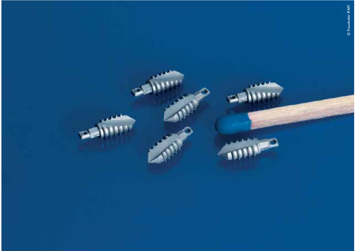
The demonstrator for a suture anchor made of iron-tricalcium phosphate (FE-TCP) is only slightly larger than a match head.
