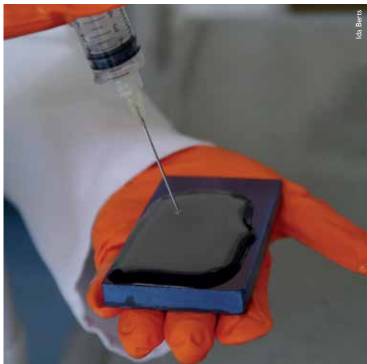
Gel coated titanium surface binds proteins which promote bone formation
