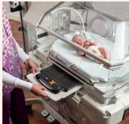
The Carestream DRX 2530C detector for paediatric imaging
