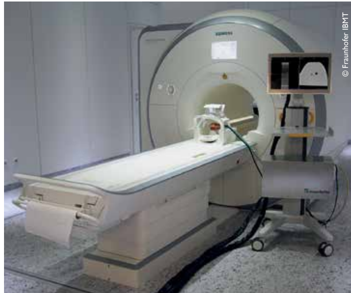
MR-compatible ultrasound research platform for multimodal imaging and a combination of the advantages of MR imaging and ultrasound imaging for ultrasound-supported movement tracking of internal organs during MRT imaging.
