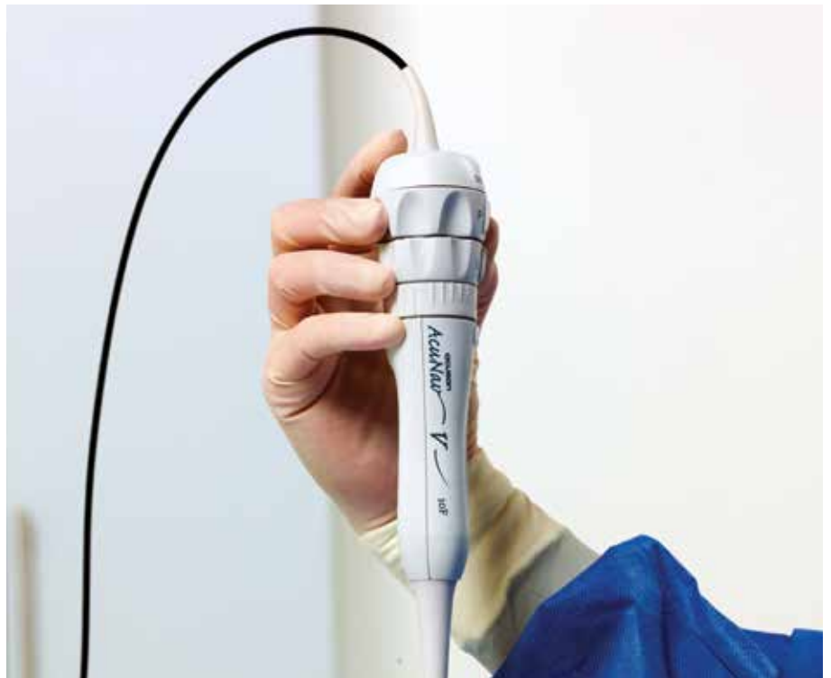
Siemens' intra-cardiac catheter
