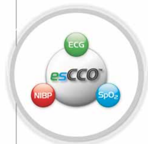
Figure 4: Principle of esCCO™. The esCCO is a new technology to determine the cardiac output non-invasively based on the Pulse Wave Transit Time (PWTT). PWTT is the time from the ECG R-wave peak to the pulse wave rise point and calculated from ECG and SpO 2 pulse waves at the fingertip. There is inverse correlation between PWTT and stroke volume, which has been confirmed by many experiments and data analysis, and has been shown to be unaffected by administration of drugs including vascular agents.
